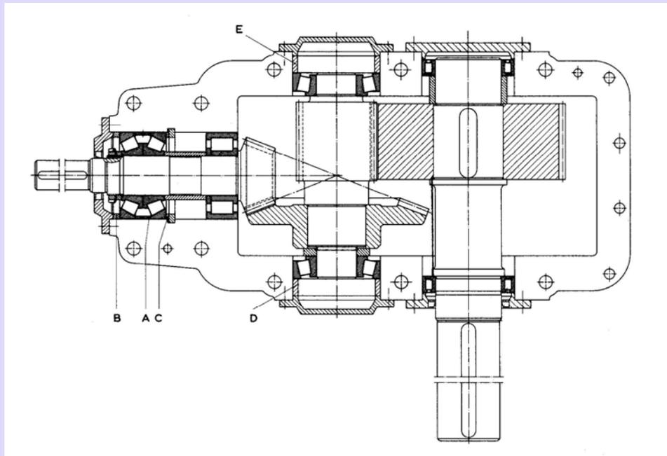
**Fig.17.10 Bevel gear – Spur gear transmission**
