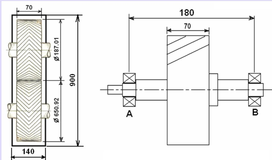
**Fig 17.18 Pinion shaft layout diagram**
