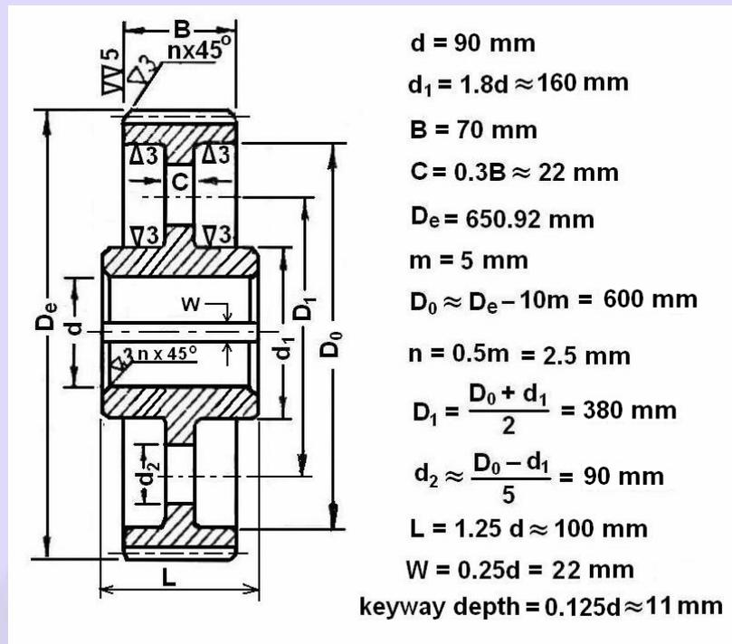
**Fig.17.27 Gear blank revised drawing showing all the dimensions.**
