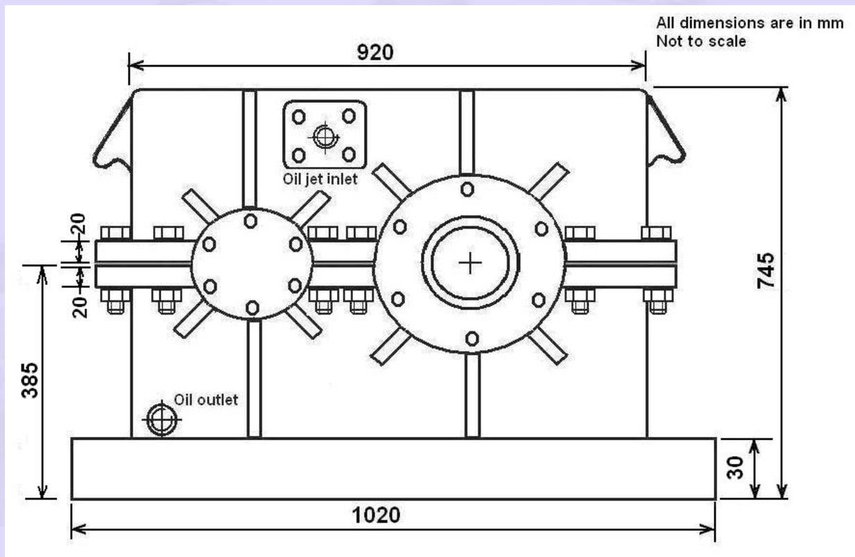
**Fig.17.28 Front view of the assembly of the gearbox**
