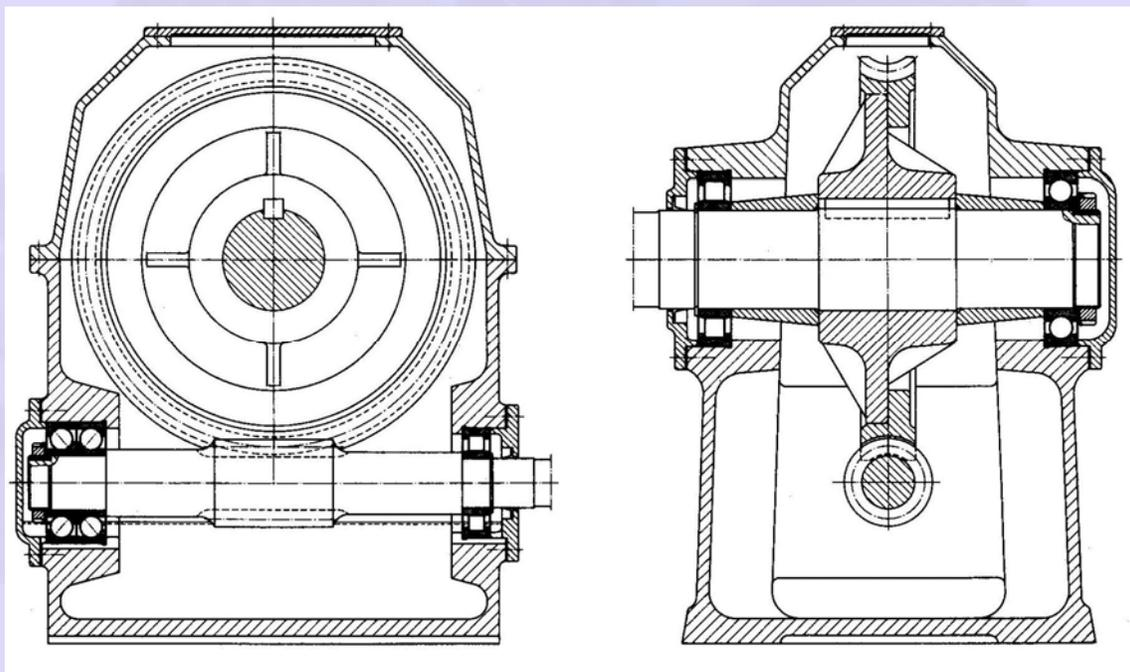
**Fig.17.6 Worm gearbox, without cooling fins, sectional front and side views**
