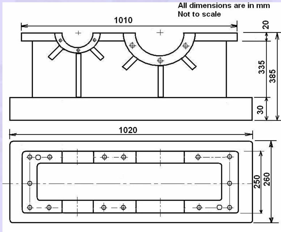
**Fig.17.19 View of bottom half of the gearbox**
