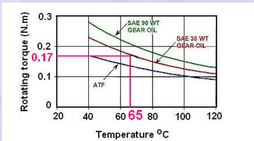
**Graph 17.23a Friction torque at various temperatures for nitrile rubber**
