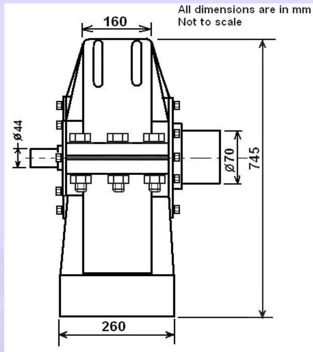
**Fig.17.29 End view of the gearbox**
