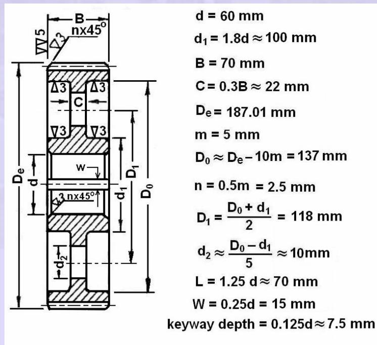
Fig.17.26 Pinion blank revised drawing showing all the dimensions
