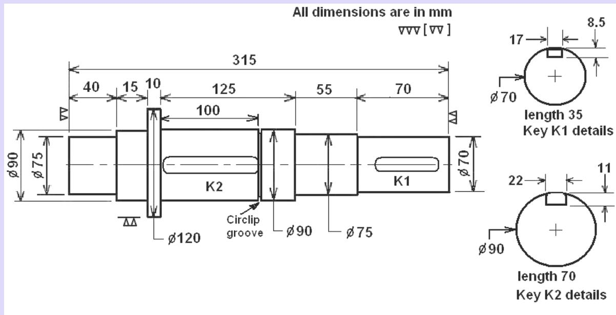
Fig.17.25 Gear shaft drawing material ductile iron 120/90/02 hardened to 331 Bhn
