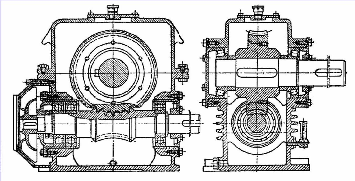
**Fig.17.5 Worm gearbox, sectional front and side views**
