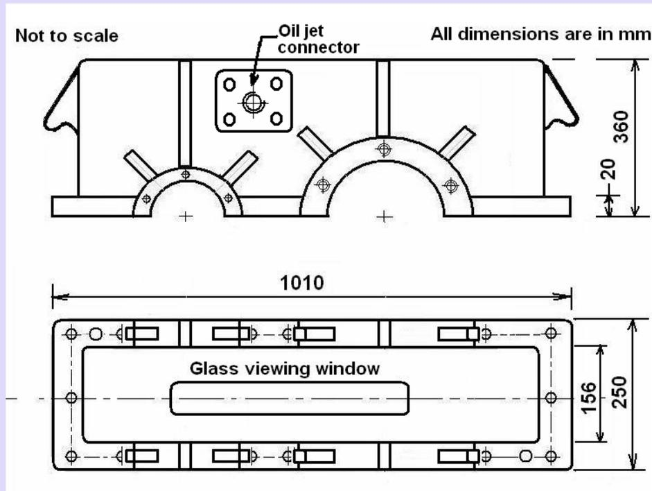
**Fig.17.20 View of top cover of the gearbox**
