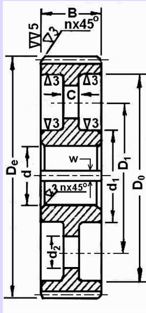
Fig.17.16. Pinion blank drawing
