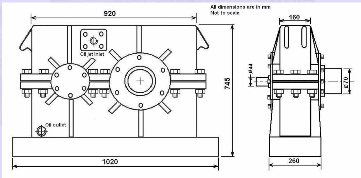
**Fig.17.30 Assembled view of the helical gearbox**
