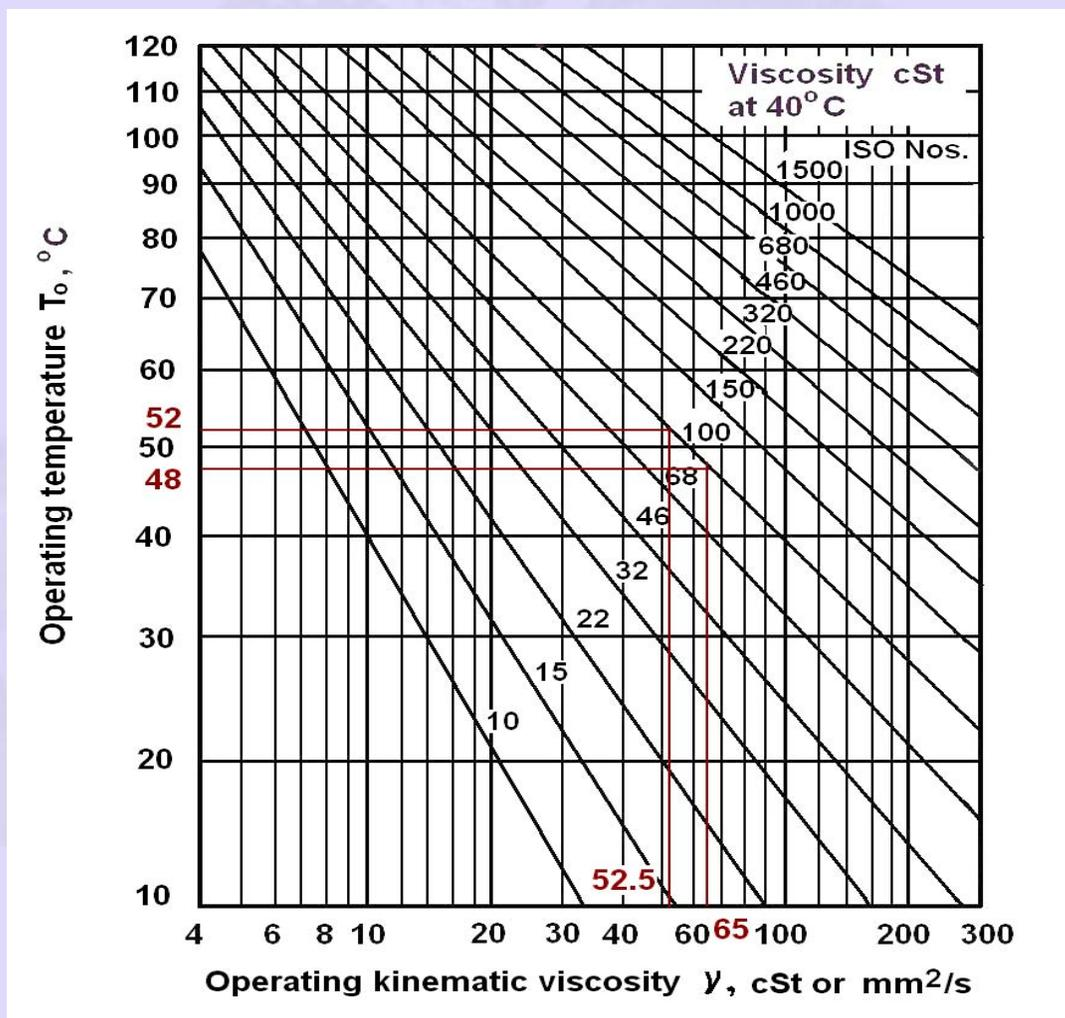
**Fig.17.21 Viscosity – Temperature curve for ISO VG graded oils**
