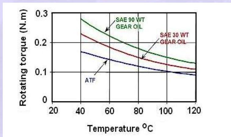
**Fig. 17.23 Friction torque at various temperature for nitrile rubber S type oil seal, Shaft diameter 50mm, speed 1000 rpm**
