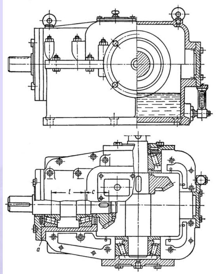
**Fig.17.3 A single stage bevel gearbox**
