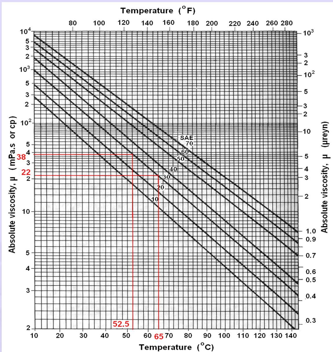
Fig.17.22 Viscosity – Temperature curves of SAE graded oils
