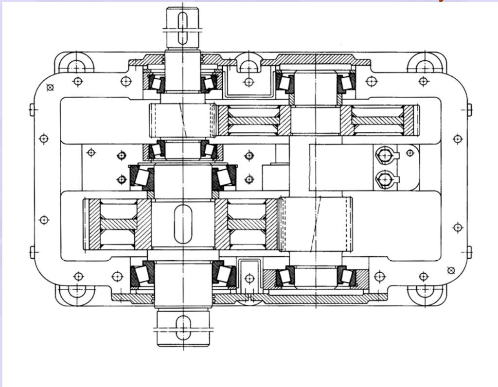
**Fig.17.9 A double reduction spur gear box**
