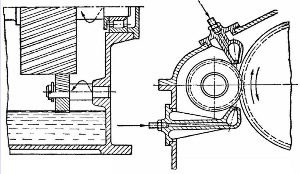
**Fig.17.7 Helical gear lubrication with idler gear**
