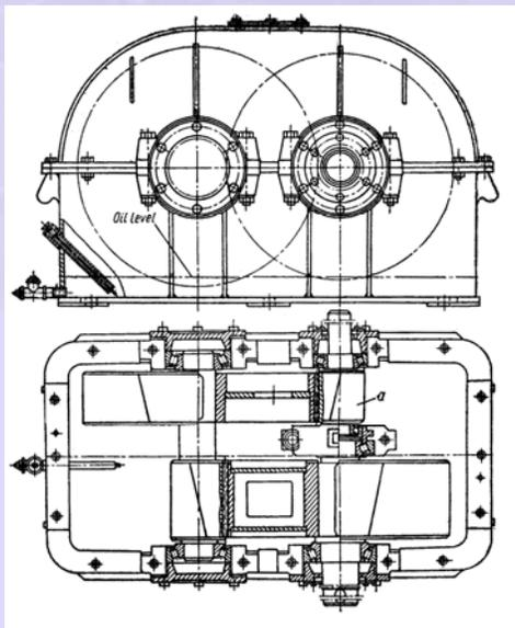
**Fig. 17.2 Two stage helical gearbox**
