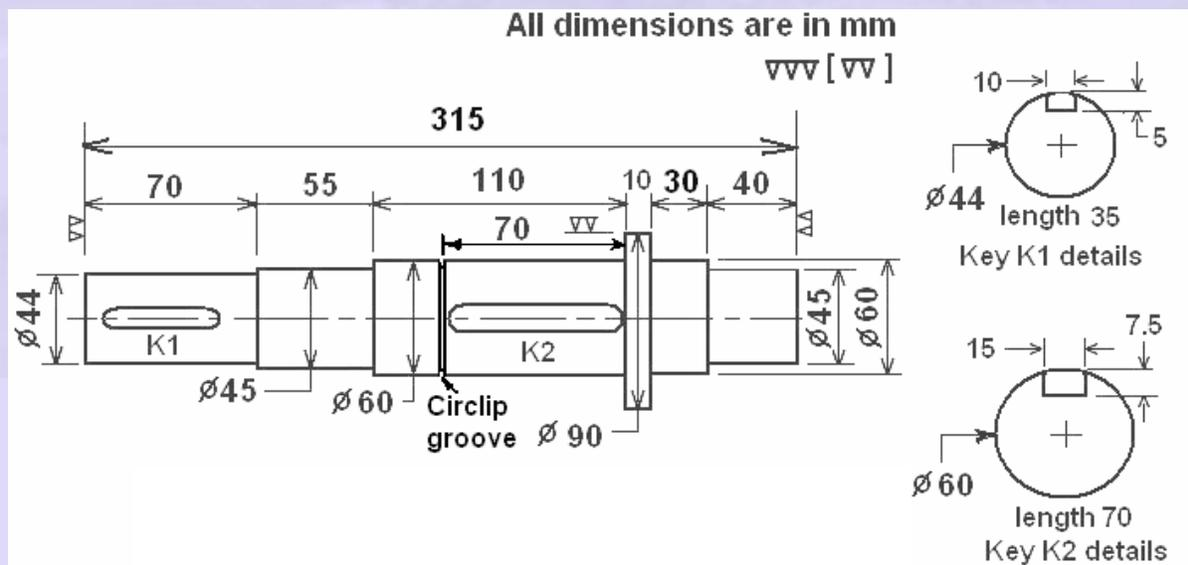
**Fig.17.24 Pinion shaft drawing material C 45 hardened and tempered to 380 Bhn**
