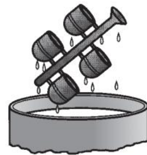
(3) the pattern tree is coated with a thin layer of refractory material
