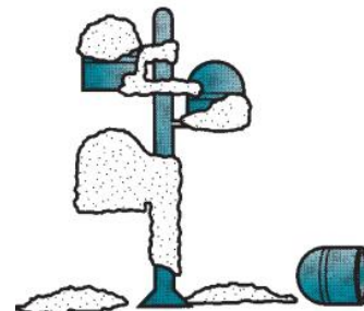
(7) the mold is broken away from the finished casting. Parts are separated from the sprue.
