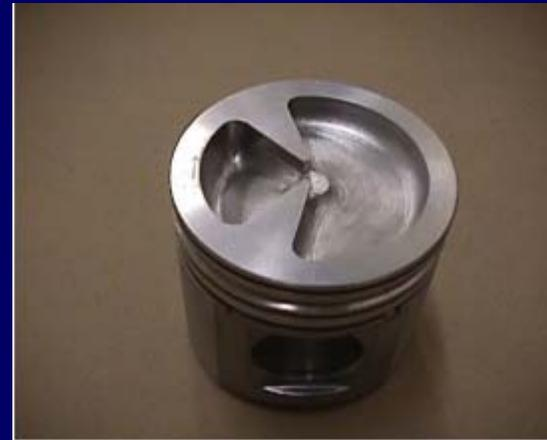
By changing the shape of the piston head, stratification is effectively produced.
