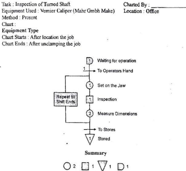
**Figure 4:** Flow Process Chart (Equipment Type) For The Inspection Of A Turned Shaft
