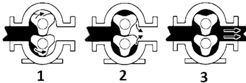
1. As the lobes come out of mesh, they create expanding volume on the inlet side of the pump. Liquid flows into the cavity and is trapped by the lobes as they rotate.
