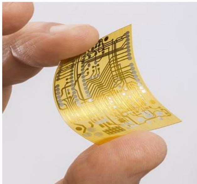
Close-up of a multilayer PCB printed by the DragonFly 2020 3D printer. Image: Nano Dimension
