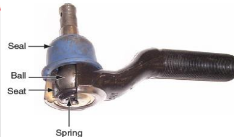
Figure 65.12 A cutaway of a tie-rod end.
